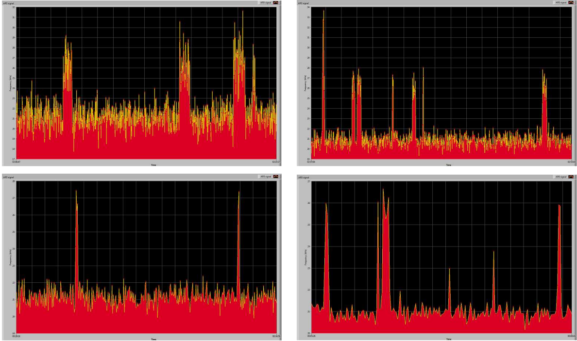
Figure 6.11: Single atom signals measured by the APD with several different integration times: 20 ms (top, left), 70 ms (top, right), 100 ms (bottom, left), and 300 ms (bottom, right). Single atom signals have good resolution in the cases of 70 ms and 100 ms.
