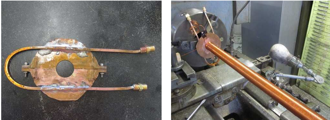
Figure 4.16: A copper plate on which a square copper tube was welded for water cooling (left). Zeeman slower winding on a lathe (right).
