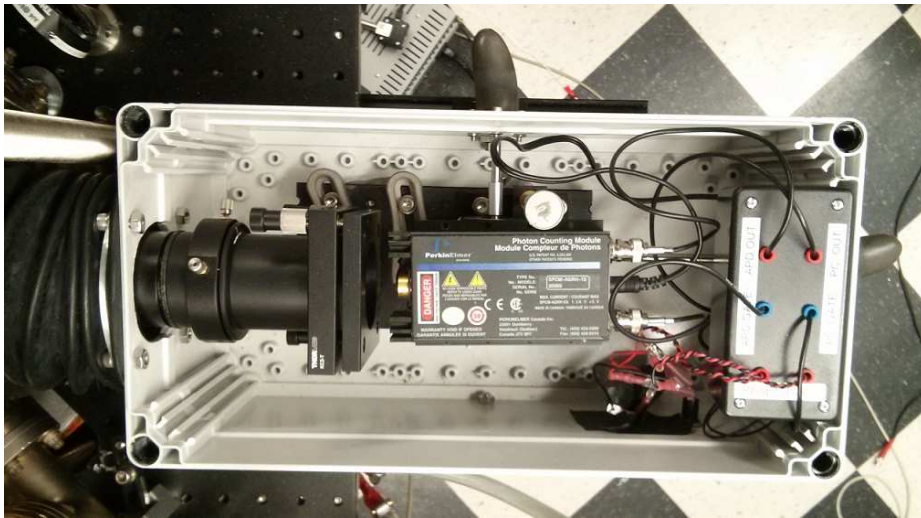
Figure 6.4: Photo of the single atom detection system.
