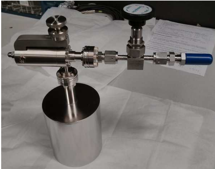
Figure 7.5: A pipette to extract and carry xenon gas from the XENON100 detector.
