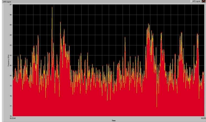
Figure 6.6: Single atom signals captured by the APD with a high background fluctuation. Our signals are \sim 5 kHz high, but fluctuation of the background noise makes it difficult to discriminate each atom.
