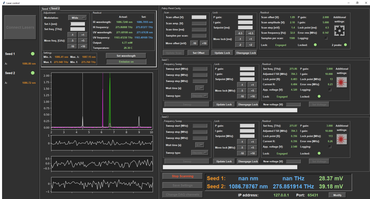
Figure 8.4.2: Screenshot of our home-built scanning cavity locking software. White peaks correspond to Cs reference laser signals, green ones are created by the rotational cooling seed laser and magenta by the detection seed laser.
