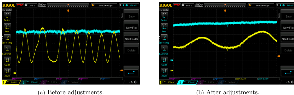
Figure 9.2.2: Photodiode signal traces taken from the oscilloscope. The cyan trace corresponds to high-power beam of polarization accepted by the doubling cavity, while the yellow trace corresponds to the low-power beam of rejected polarization. Before adjustments were made, oscillation period was about 1 min (one box corresponds to 50 s), while after it is as long as 6 min. The amplitude decreased by a factor of 2.
