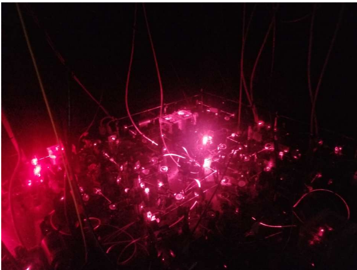
Figure 3.14: I show an image of the laser table where the detection, cooling, and repumping light is generated before it is coupled to single mode fibers to be transported to the experiment table.
