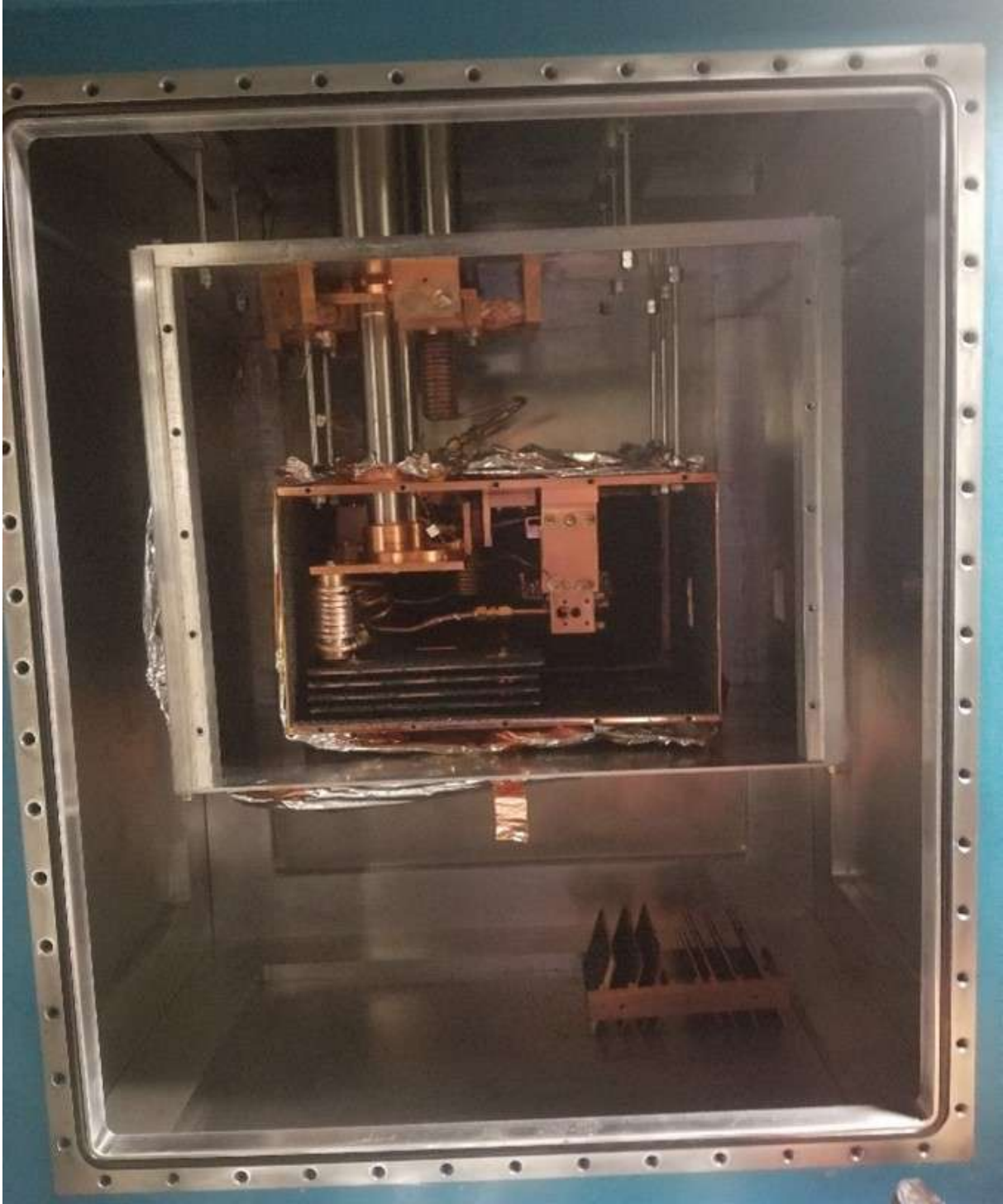
Figure 3.4: I show all the layers of the cryostat after we opened the system for cell maintenance. The room temperature shield can be seen on the outer edge along with the rubber gasket which provides the air-tight seal. A bank of cryogenic charcoal sorb fins can be seen resting on the base of the room temperature shield. Within , the aluminum 40K shield can be seen encasing the copper 4K region. Within, the 4K region one may observe the 4K PTR head, the ablation cell, the helium buffer gas bobbins, and additional charcoal sorbs.
