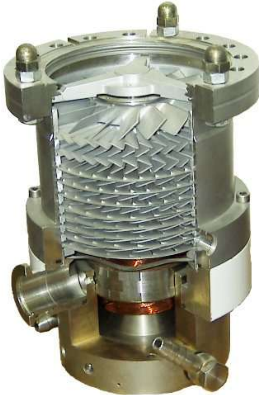
Figure 3.9: I show a cross section of a turbo pump. One may observe the many layers of turbo fans that change angle to gradually force gas out from the vacuum system through the flange on the bottom left. [157]
