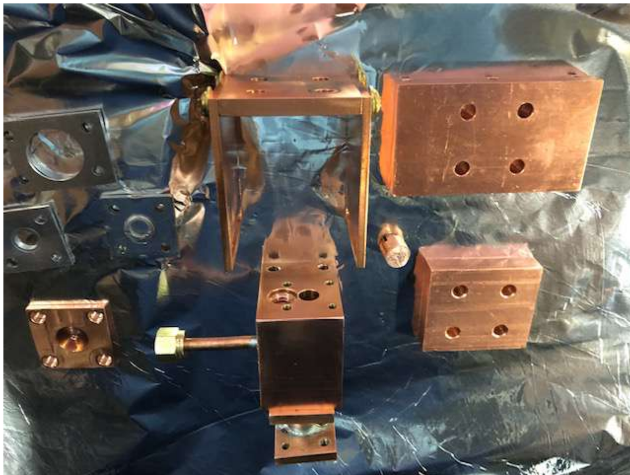
Figure 3.6: I show the components of the cell assembly after it was taken out of the cryostat. I show the cell, the cell windows, the cell aperture, the sample holder, and the thermal coupling plates.
