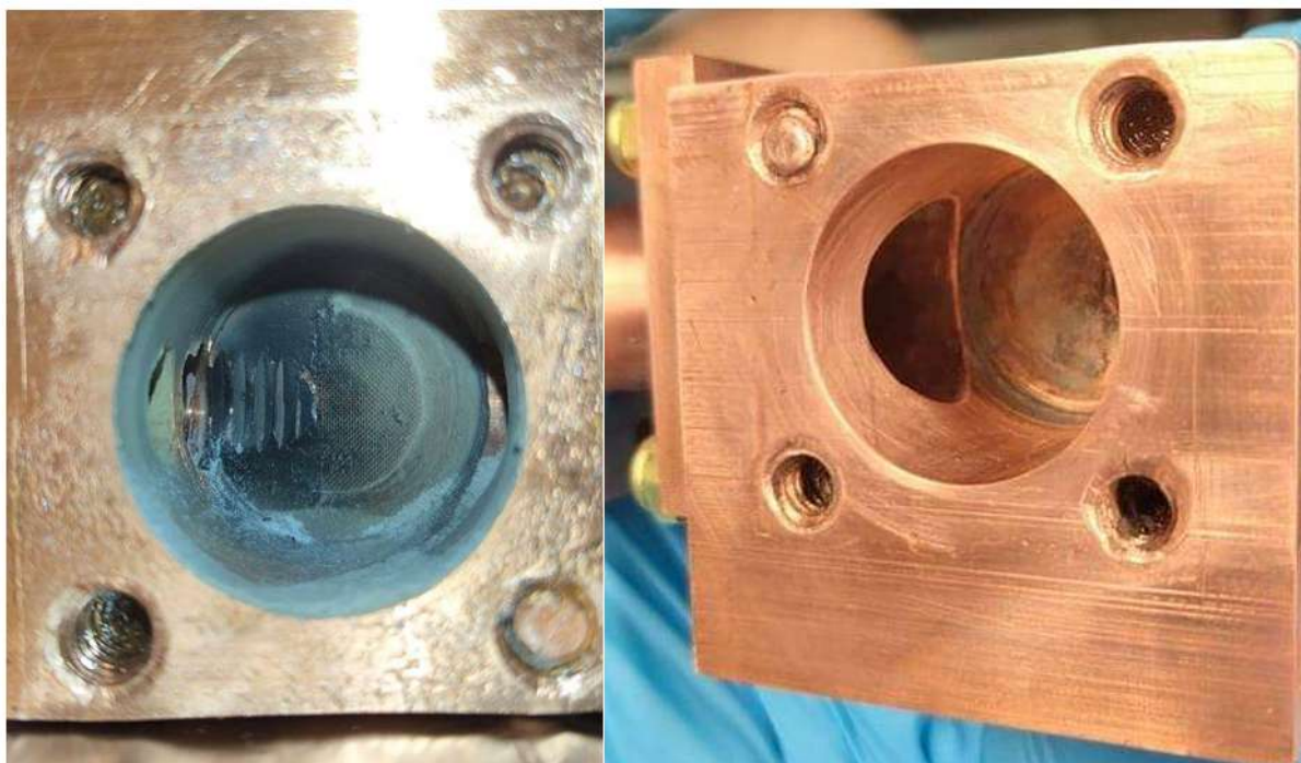
Figure 3.8: On the left, I show images of a cell after weeks of ablation. The powder seen at the bottom of the cell is debris blasted off the sample by the focused ablation laser. On the right, I show the cell after we sanded it and destroyed the beam.
