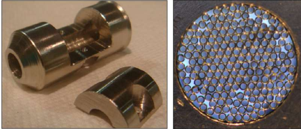
Figure 2.7: Microtube holder, before assembly (left). Cross-sectional photograph of the assembled microtubes in the holder (right).
