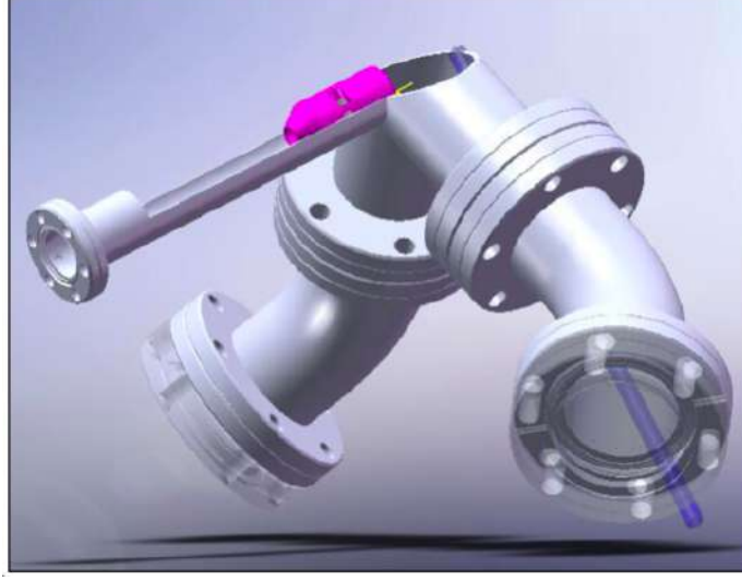
Figure 2.5: Rendering of the oven design, assembled with the fitted microtube holder.
