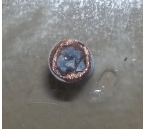
Figure 3.6: Example image of the BaH targets ready to be loaded into the cell. Note that slight "shine" caused by glue wicking up the sides of the targets. We found this greatly improved the lifetime of the sample during sustained ablation.
