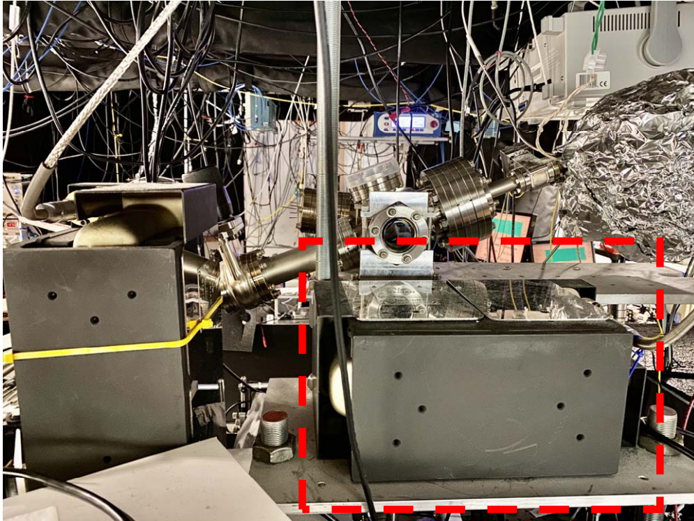
Figure A.4: The ion pump circled in dashed red line takes care of the region before the chamber valve. On the left side of this figure is another ion pump, which takes care of the Zeeman slower tube area.
