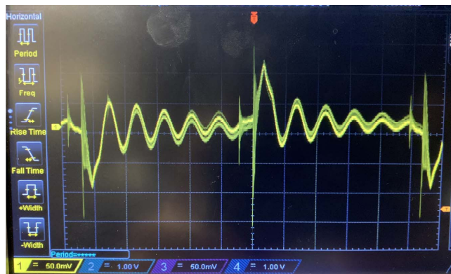
Figure A.5: The vacuum status can be monitored with high sensitivity from the ion pump voltage output reading. The vacuum level is indicated by the offset of the voltage output.
