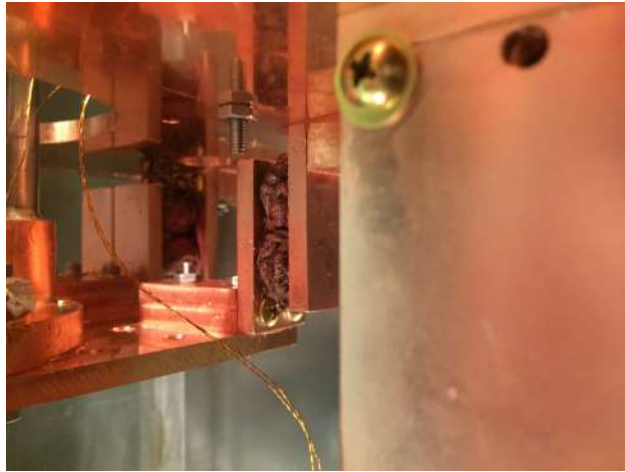
Figure E.2: Copper rope lug for thermal connection on the 4K stage.
