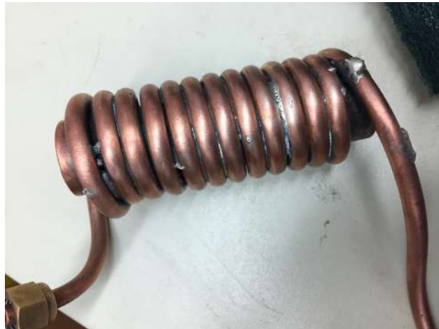
Figure E.5: Soldered copper bobbin for He gas thermalization.
