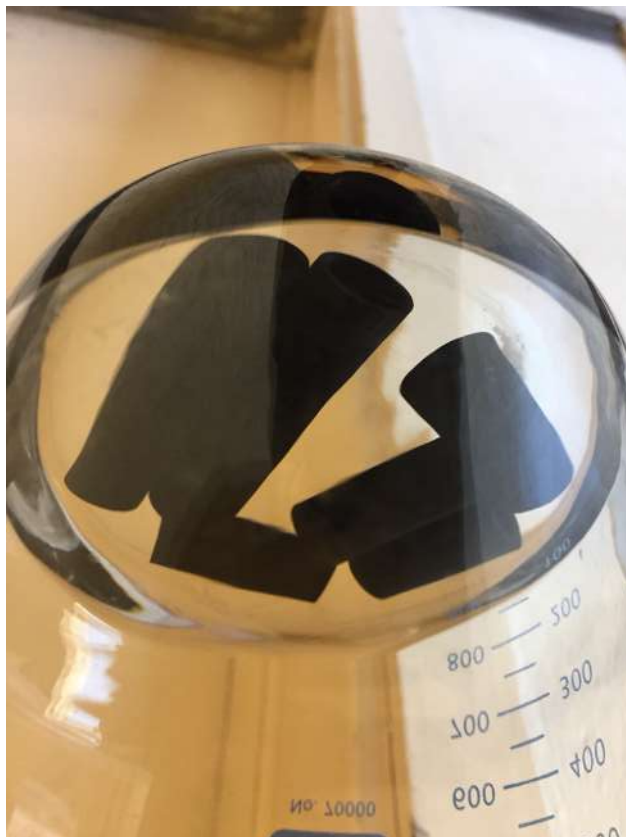
Figure 4.16: Photo of blackened OFHC copper pipe-baffles used in the octagonal detection region. Here, there are shown just after blackening, being rinsed in deionized water.
